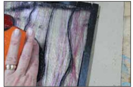
The frit should be approximately up to the level of the other glass. Have it completely cover the Nichrome 60 wire.
