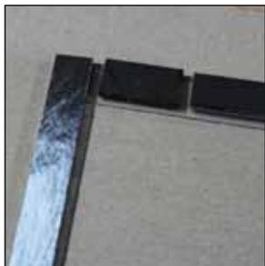
The strips can be pieced together to line the sides of the panel, but be certain to leave small gaps at the tops of the panel on the right and the left for insertion of the hanging wires. The rest of the black strips should touch and not have any gaps. Adhere the strips with small dots of Super Glue. Remember to check that the iridized glass is irid side up, if you’ve chosen that.
