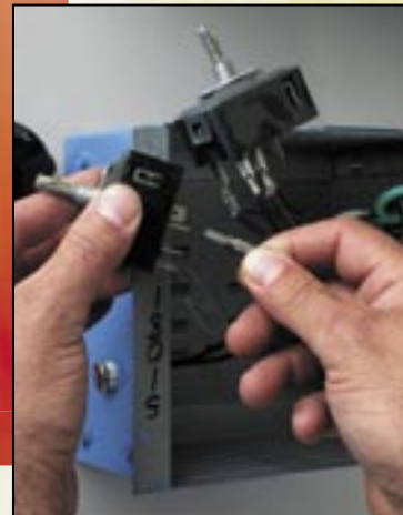
Firefly switch replacement C1. Make sure the connections are tight when you replace electrical components.
