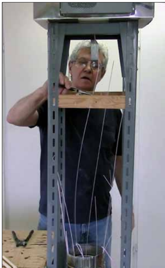
Kiln with stand bolted to a 6-foot-tall metal angle bar. Dropping a stream of glass into a stovepipe is a great way to make long, straight stringers.
