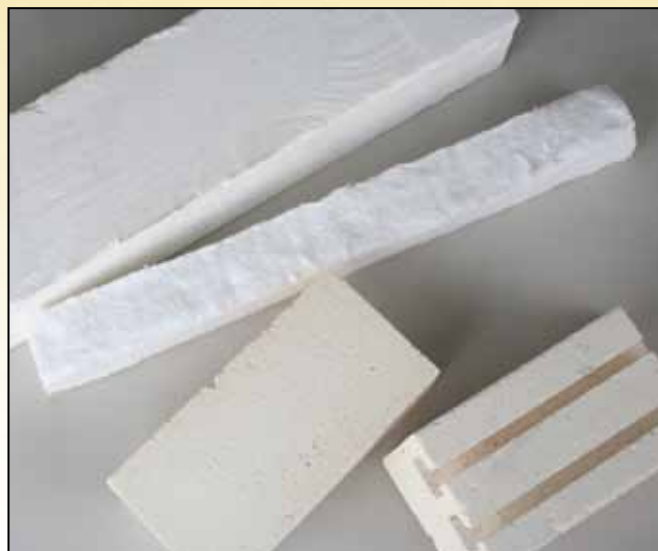
Kilns are insulated with either ceramic fiber or insulating firebricks. Ceramic fiber heats and cools more rapidly than firebricks, while a firebrick kiln is more suitable for long annealing times.
