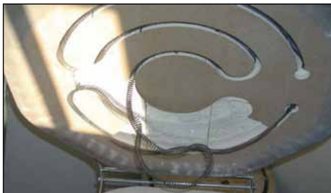
Collapsed kiln lid caused by thermal shock
