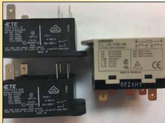
*Read the label printed on the side of the relay and compare it to the label on the relay you are replacing.*
