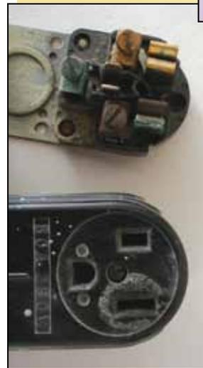
If the wall receptacle feels unusually warm or smells like burning plastic, disconnect the circuit breaker and have the outlet serviced. Loose connections can cause the outlet to overheat, which is a fire hazard.
