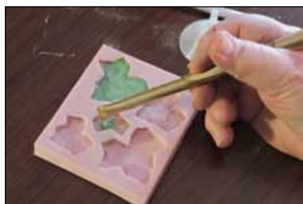
Using a powder vibe to fill molds with dry glass powder
