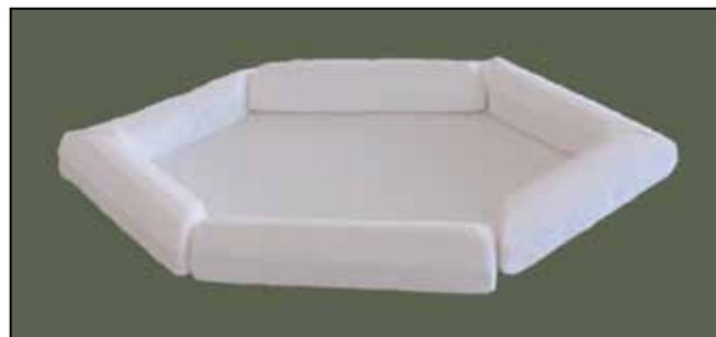
This 1" x 6" x 6" setup was made with 1-1/2" Kaiser Lee Boards.
