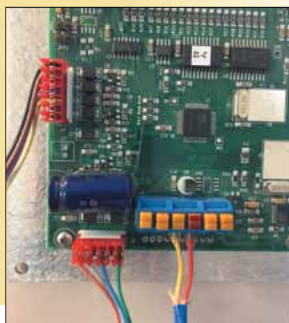
This shows the back of the temperature controller. The thermocouple wires are at the bottom right of the photo. They give the controller a continuous temperature reading from the firing chamber.
