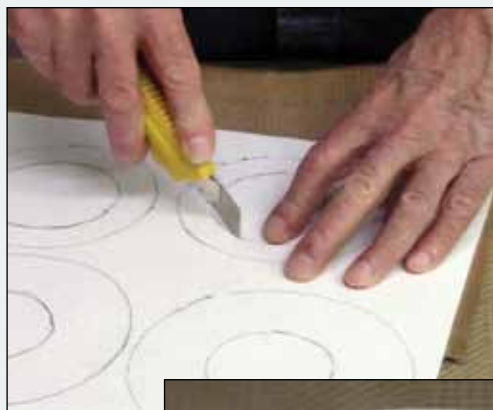
Cutting out fiber paper to make the slump mold
