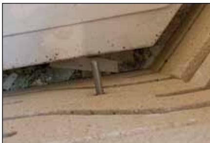
The thermocouple is the small rod that extends into the firing chamber. On the other side of the kiln wall you will find a control panel or switch box. Remove that panel.
