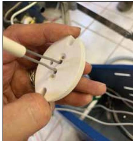
Turn the connection block over and look at the side that goes toward the kiln wall. You will find two pins. If those pins extend past the ceramic block, they could touch the kiln case and short out the thermocouple. It would still work, but with reduced accuracy. If the pins extend past the oval block surface, replace the block.
