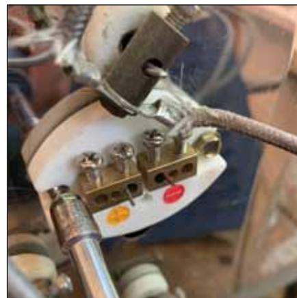
Label the four wires on the connection block so you can reinstall them correctly later. Two screws attach the thermocouple connection block to the kiln. Remove those two screws as shown and gently slide the thermocouple out of the kiln for further examination.
