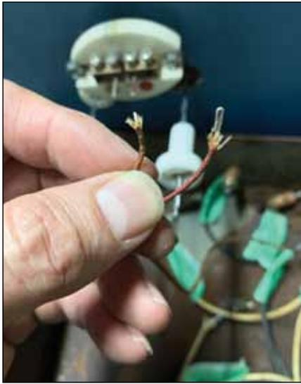
When I removed the thermocouple-to-relay wires on a kiln I was repairing, I found that the wire on the left had been broken due to excessive pressure from a screw. This type of damage can be seen by removing the wires.
