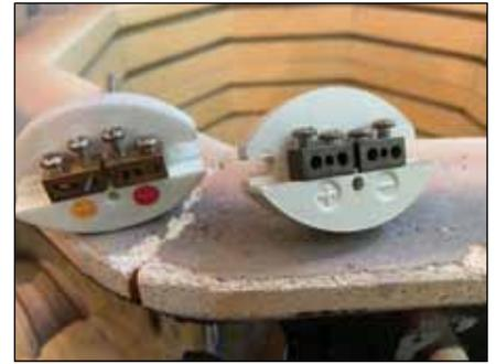
The thermocouple connection block shown here on the left is new. The one on the right is tarnished. Replace the connection block if it's tarnished or clean out the holes where the wires go. Clean and reinstall the wires on the connection block.
