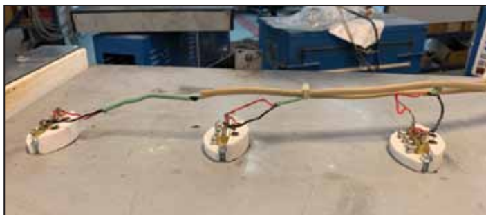
(Photo 1) The thermocouples are mounted in the top of a kiln. The steel they were mounted on moved upward and caused a thermocouple to touch the top panel (removed for the photo). This threw off the temperature reading.
