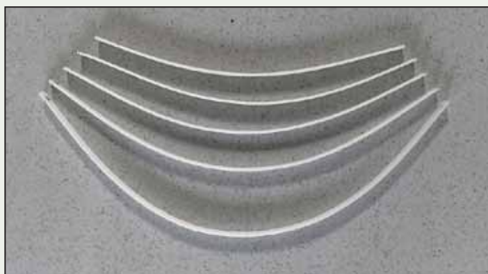
(Figure 1) Strips of varying lengths of white glass were slumped simultaneously. The strips with the greatest span slumped the most.
