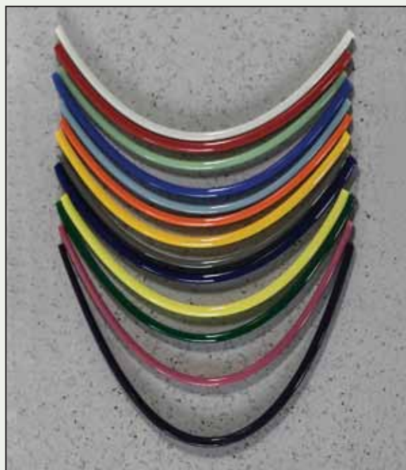
(Figure 3) Glass rods of equal length have been slumped simultaneously to the same temperature. The stiff, viscous colors have slumped less than the soft, less viscous colors.
