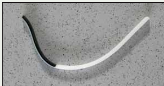
(Figure 4) The variation in viscosity from soft black glass to stiff white glass results in a lopsided slump.
