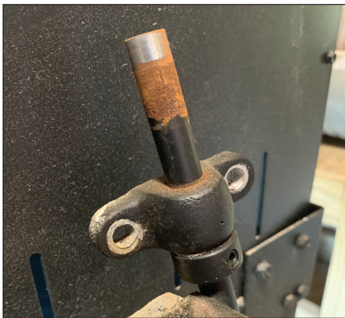
This kiln is newer than the ones in the other photos. It shows the top of the hinge shaft after I removed the door. The pillow block shown here was so corroded that I had to cut it off with a hacksaw.
