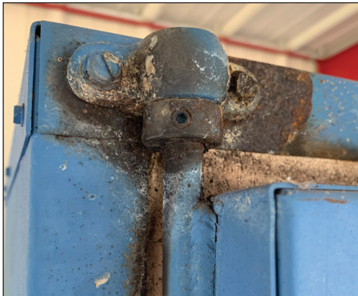
This top pillow block has 16 years of corrosion. Notice how the weld on the door shaft was beginning to crack because the door was difficult to open and close.
