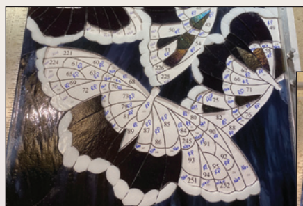
Assemble the glass pieces together.
