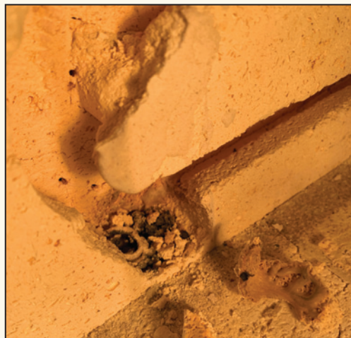
(Photo 4) After removing an element, I found particles from a previous element that had been left in the groove. You can see coils from the previous element in the photo. Always take the time to dig out metal particles, glass, or darkened areas of the groove before installing new elements.
