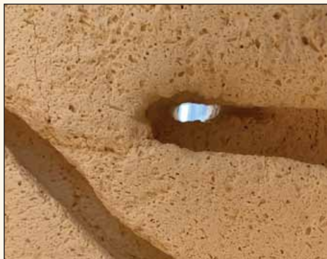
(Photo 8) This is the firebrick hole where the element goes through the kiln wall. If the hole is enlarged, heat will build up inside the kiln's switch box, causing the element connectors to become too hot and fail prematurely. An enlarged hole is usually oval shaped like this one.
