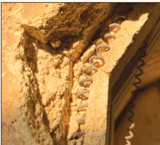
(Photo 5) The element here is half buried in firebrick particles. This reduces the heating capacity of the elements and slows down the kiln. Occasionally vacuum the firing chamber. Always wear a dust mask when vacuuming your kiln. Keep the vacuum nozzle away from the thermocouple and controller to avoid damage from static electricity.
