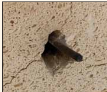
(Photo 1) Notice how large the hole is where the thermocouple enters the firing chamber. The gap around the thermocouple allows air to change the accuracy of the temperature reading. The thermocouple should have a snug fit. The hole in this picture may have held a wider thermocouple that was replaced with a thinner one.
