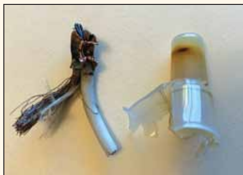
(Photo 3) After I replace a part, I often cut it open to find out what caused it to fail. In this case, the insulation from the thick wire on the right was up inside the brass connector barrel, creating a gap that prevented a good connection between the wires. You can see the heat damage on the nylon cover.
