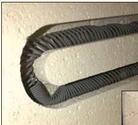
(Photo 6) Notice how the element coils have bunched up in the bottom of the groove where it curves in front of the kiln door. Bunched element coils get too hot. You can reduce this by inserting three evenly spaced element pins in the curve.
