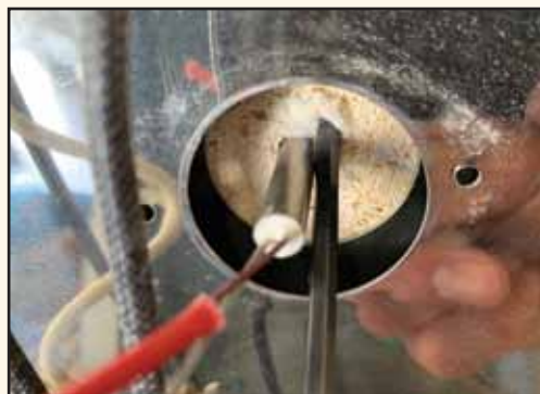
(Photo 2) You can stuff an enlarged thermocouple hole with ceramic fiber to prevent the flow of air around the thermocouple.
