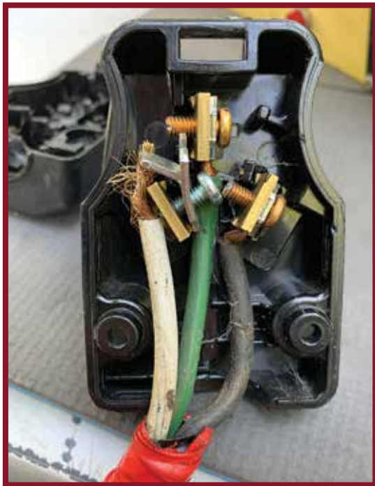
This is exactly the way I found the inside of a kiln plug. Be extremely careful in wiring anything on a kiln.
