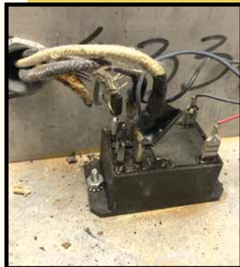
Loose relay wires.
