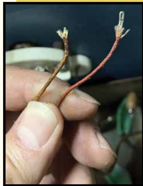
Broken thermocouple wire.
